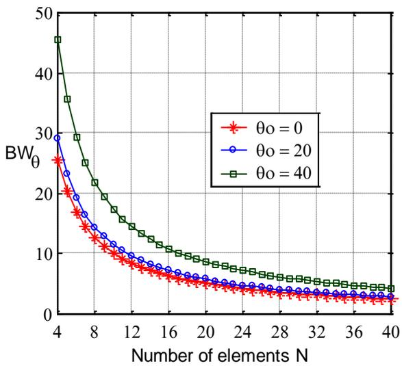
Fig. 5  $BW_{\theta}$  in degrees versus number of elements ( $N$ ) at different beam orientation angle  $\theta_o$
