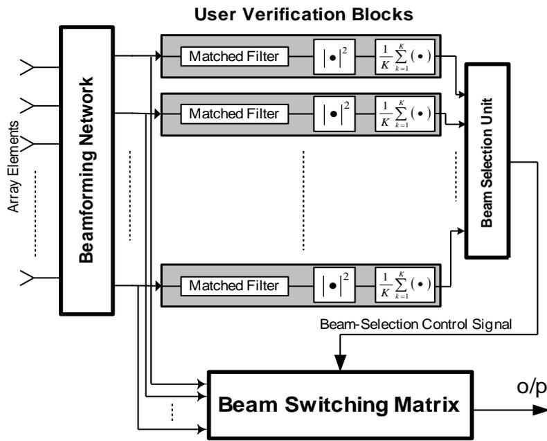
Fig. 1. General switched-beam system
