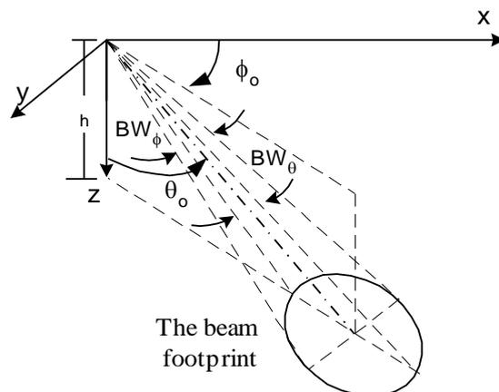
Fig. 4 The beam footprint and beamwidths
