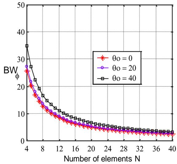
Fig. 6  $BW_{\phi}$  in degrees versus number of elements ( $N$ ) at different beam orientation angle  $\theta_o$
