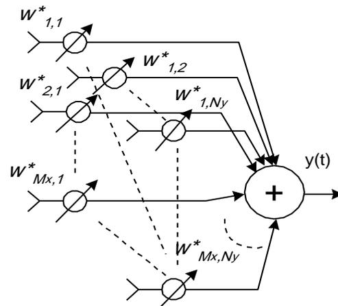
Fig. 3 Two-dimensional antenna array beamformer
