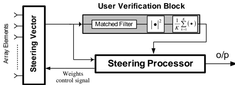
Fig. 7 The block diagram of the single-scanning beam switching system
