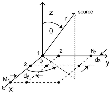
Fig. 2 Two-dimensional antenna array
