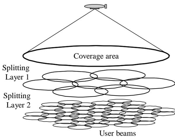
Fig. 8 Beam-splitting for user acquisition
