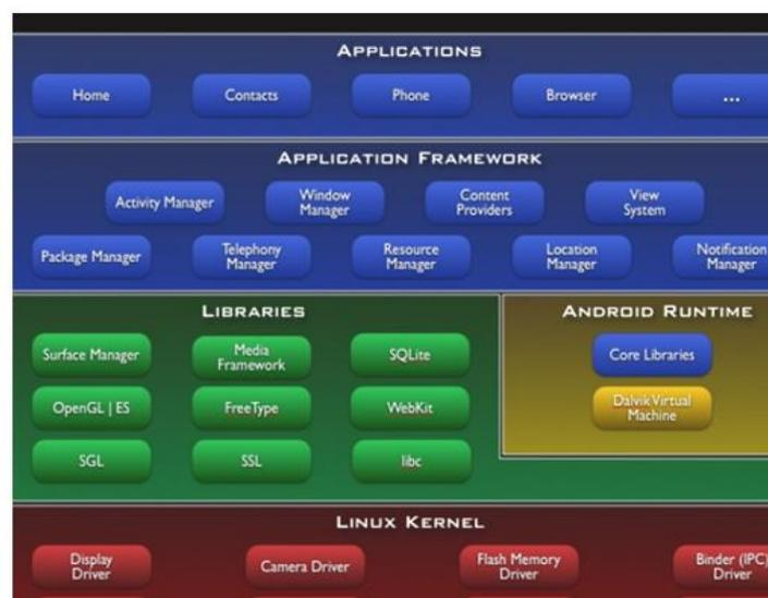
Figure 1 Android’s four-layer model [2]
